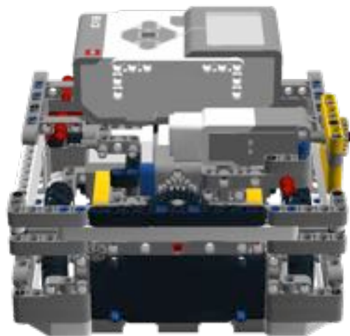
front view of the robot. Including the addition of the side facing medium motor
